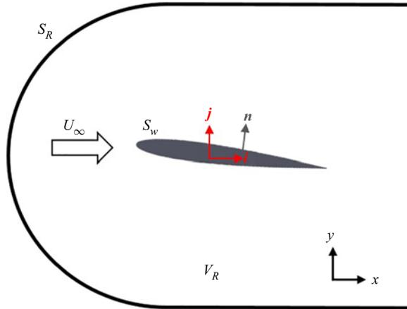
Figure 1. Schematic showing the configuration of vorticity force analysis, where  $V_R$  is the control volume,  $S_w$  is the surface of the aerofoil,  $S_R$  is the cuboid surface of the control volume,  $U_\infty$  is the free stream velocity,  $\mathbf{n}$  is the normal vector of the aerofoil, and  $\mathbf{i}, \mathbf{j}$  are the unit vectors in the drag and lift directions, respectively.
