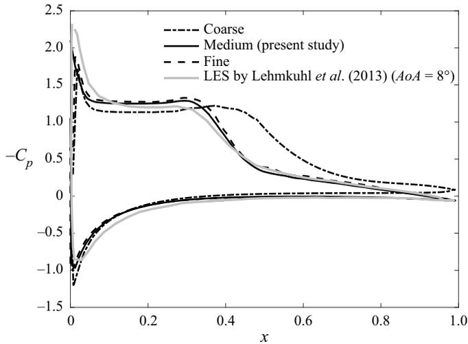
Figure 6. Distributions of the pressure coefficient ( $C_p$ ) on the surface of the NACA0012 aerofoil in the case with  $AoA = 7.5^\circ$  obtained from the present simulation with coarse (black dash-dotted line), medium (black solid line) and fine (black dashed line) grid resolutions, and the LES by Lehmkuehl *et al.* (2013) using the QR eddy-viscosity model (grey solid line).
