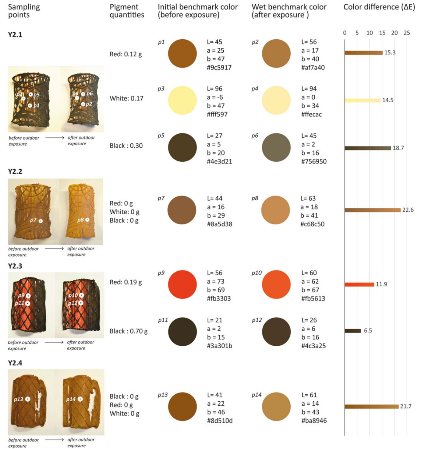
Figure 14. Chromatic shifts in robotically 3D printed YCBH samples after outdoor exposure.
