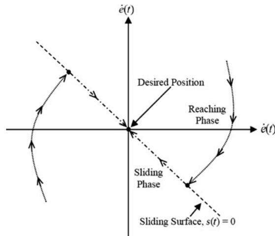
Fig. 5. The general structure of SMC.<sup>64</sup>
