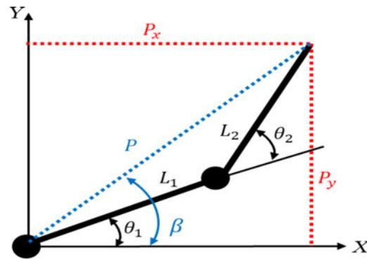
Fig. 6. A schematic of a rigid link manipulator.
