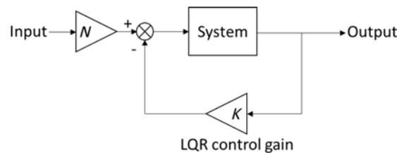
Fig. 2. LQR controller diagram.
