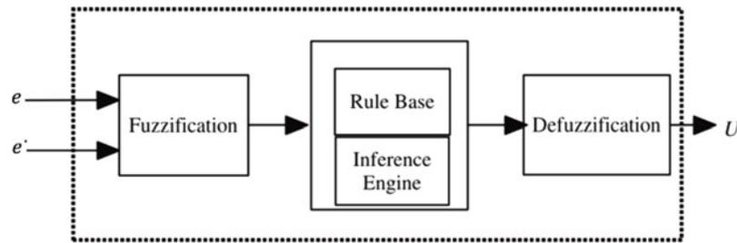
Fig. 3. Fuzzy logic controller architecture.<sup>36</sup>
