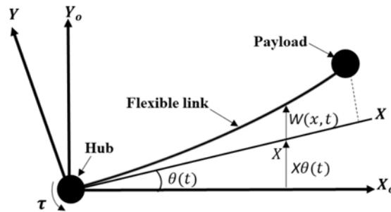
Fig. 1. The schematic diagram of the flexible link manipulator.
