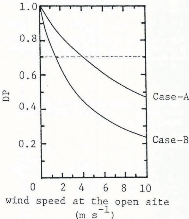
Fig. 6. Changes of  $DP$  with wind speed at the open site under a fixed relative ratio for wind speed (simulation 1).
