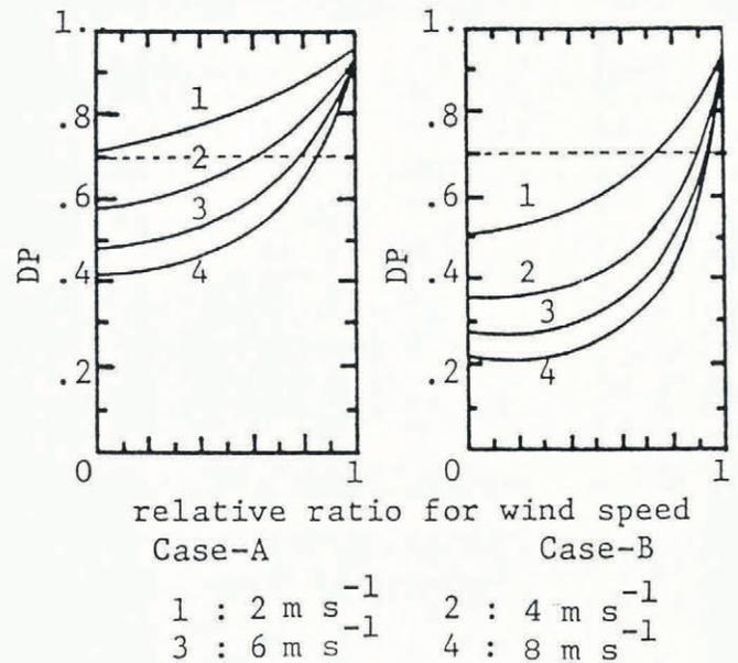
Fig. 7. Changes of  $DP$  with relative ratio for wind speed under constant wind speed at the open site (simulation 2).
