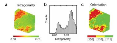
**Figure 2.** (a) The intensity map of "tetragonality" calculated from each diffraction pattern collected on the cathode NP shown in Fig. 1. (b) The histogram of "tetragonality" derived from (a). (c) The phase orientation map determined from the intensity map of "tetragonality". "t" and "c" stand for tetragonal phase and cubic phase, respectively.
