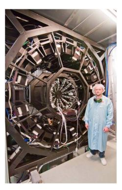
**Figure 12.** The final amplifier of POLARIS (picture courtesy of Helmholtz Institute).
