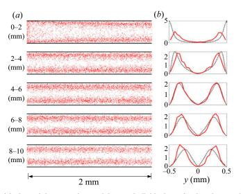
Figure 5. (a) Empirical reactivity map where red dots are individual reaction locations, and (b) the empirical PDF of y-coordinates of reaction locations in the first 1 cm channel segment at  $Pe = 10^2$ . The analytical prediction (black dashed lines) captures the simulation results near the injection location.
