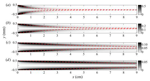
Figure 6. Reactivity maps (4.14) according to Pe in a straight channel flow. The dashed lines are the characteristic depletion location,  $x_R(y)$ . The active reaction zones upstream are near the wall and move towards the channel centre on moving downstream. (a)  $Pe = 10^2$ ; (b)  $Pe = 10^3$ ; (c)  $Pe = 10^4$ ; (d)  $Pe = 10^5$ .
