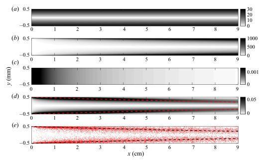
Figure 2. (a) Eulerian stretching map,  $S_E(x)$  (3.5). (b) Lagrangian stretching map,  $S_L(x)$  (3.11). (c) Analytical reactivity map for Poiseuille flow. (e) Reaction locations simulated by the RWPT method. The analytical reactivity maps and the numerical results are obtained for  $Pe = 10^5$  and  $w_0 = 5$  mm. The dashed lines are the characteristic depletion location,  $x_R(y)$  (see § 5.2).
