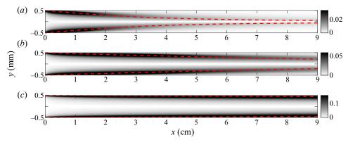
Figure 7. Reactivity maps (4.14) for the three different values of  $w_0$  in a straight channel flow. The dashed lines are the characteristic depletion location,  $x_R(y)$ . As the mass limitation is eased (as L increases), the active reaction zone stays near the channel wall, where fluid stretching is stronger, for longer distances. (a)  $W_0 = 1$  mm; (b)  $W_0 = 5$  mm; (c)  $W_0 = 10$  mm.
