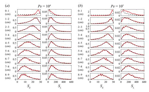
Figure 8. Empirical PDFs of Eulerian and Lagrangian stretching values sampled from reaction locations for (a)  $Pe = 10^4$  and (b)  $Pe = 10^5$  for the straight channel. The black dashed lines are analytically computed reactivity-weighted PDFs of fluid stretching (5.9). The observed stretching–reactivity relations demonstrate that there exist optimal ranges of fluid stretching for high reactivity.
