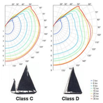
*Figure 13.* Polar diagram of vessel speed in relation to wind speed and wind angle – for yachts. (Żegluj.net, 2014).
