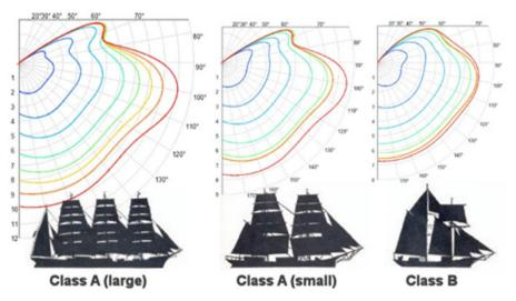
*Figure 14.* Polar diagram of sailing vessel speed in relation to wind speed and wind angle – for sailing vessels of varied sizes (Żegluj.net, 2014).
