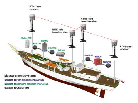
Figure 16. Location of the measurement apparatus on the Dar Młodzieży sailing vessel.
