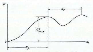
Fig. 4. Graph of approximate dependence of  $\Phi$  on limiting length of snow transport  $x_1$ .
