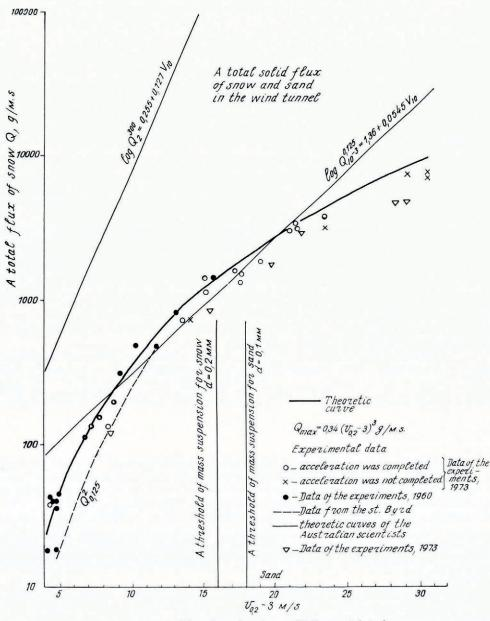
Fig 1. Graph of dependence of maximum solid flux on wind speeds.
