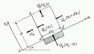
Fig. 3. Theoretical model of snow-storm on a mountainous slope.
