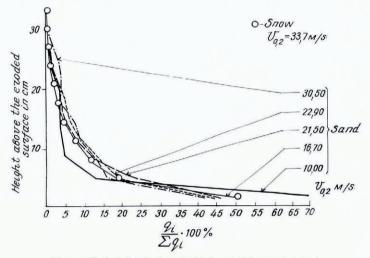
Fig. 2. Vertical distribution of solid flux at different wind speeds.
