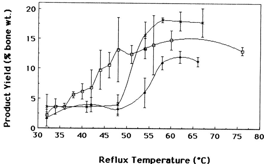
Fig 1. Variation of product yield with reflux temperature for samples A (X), B (♦) and C (□). The error bars represent the one standard deviation scatter in the five subsamples processed at each reflux temperature.
