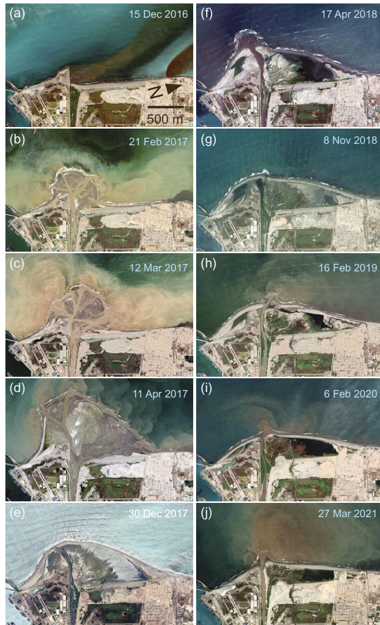
Figure 1. The influence of river sediment discharge on the coastal morphology and shoreline positions at the mouth of Rio Rimac, Peru, from 2016 to 2021. As described by Guzman et al. (2020), heavy flooding in early 2017 resulted in massive growth of the river mouth delta and spreading of this sediment northward in the subsequent years, similar to the coastal morphodynamics following flooding in 1983 and 1998. Imagery from Google Earth.
