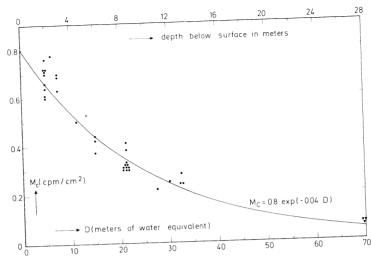
Fig 3. Meson counting rates of a number of  $^{14}\text{C}$  proportional counters per cm $^2$  of effective counter cross-section as a function of the shielding. The shielding capacity of sand and concrete was transferred to meters of water equivalent by using an average specific gravity of  $2.5\text{g/cm}^3$ . The shielding effect observed is 4%m of water or ca 10%m of depth (Eq 4).
