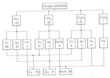
Fig 1. Survey of construction materials and counting gases used for  $^{14}$  C proportional counters. This compilation represents > 80% of the  $^{14}$ C counters in operation. Cu = copper, Ou = quartz, Fe = iron, Ni = nickel.
