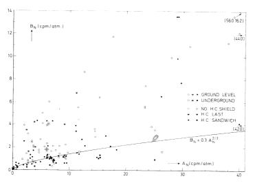
Fig 5. Relation between  $^{14}$ C counter background,  $B_N$ , normalized to 1 atm (Eq 6) and the effective counter size, represented by the normalized standard activity,  $A_N$  (Eq 1). Identifications are made of the position of the counter with respect to ground level (underground = > 7m below ground level) and type of shielding.
