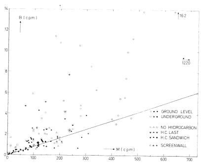
Fig 4. Background counting rate (B) as a function of meson counting rate (M). The underground laboratories (below 7m) are specifically indicated. Further identification was made for Oeschger-type counters and for the counter shielding: no neutron shielding by a layer of a hydrocarbon compound (HC), merely an inner layer of HC and a layer of HC between two layers of high specific density material (HC sandwich). The solid line indicates a favourable trend of B/M of 0.83% (2.5cpm/300cpm).
