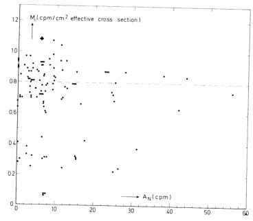
Fig 2. Meson counting rates of  $^{14}\text{C}$  proportional counters per cm $^2$  of effective counter cross section (Eq 3) as a function of the effective counter size (normalized standard counting rate (Eq 1)). The triangular points are maximum counting rates.
