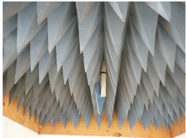
Figure 2. Pyramidal foam absorber with log-periodic dipole array (LPDA) reference antenna located at centre. The absorber is housed in a metal-backed wooden box.
