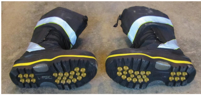
Fig. 6. No noticeable effect on boot soles after 2 weeks of exposure to ESTISOL™ 140 at ABN.
