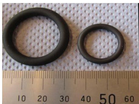
Fig. 4. O-ring after immersion for 2 days (right); O-ring with no immersion (left).
