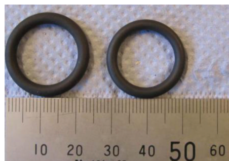
Fig. 5. O-ring returns to approximately original dimensions after 7 days at room temperature (right); O-ring with no immersion (left).
