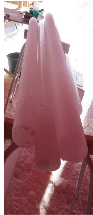
Fig. 7. First ice cores to be drilled using ESTISOL™ 140 giving consistently good-quality ice cores.
