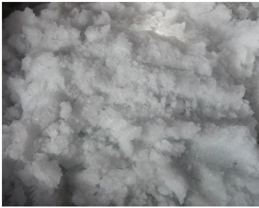
Fig. 8. Drill chips collected at 125 m: good chip size (~2–3 mm) and recovery.
