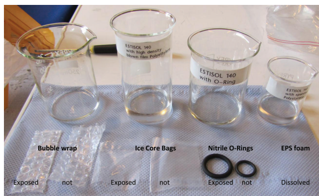
Fig. 3. A selection of the materials tested by immersion compared with no immersion.
