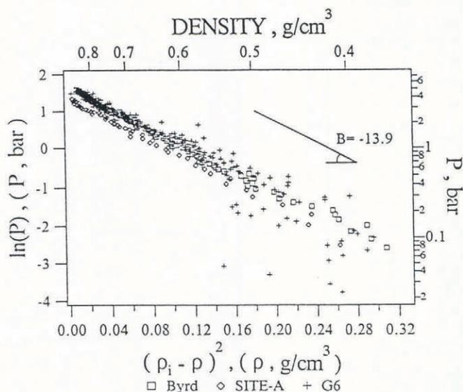
Fig. 7. Relationships between overburden pressure and density at Byrd, G6 and site A.
