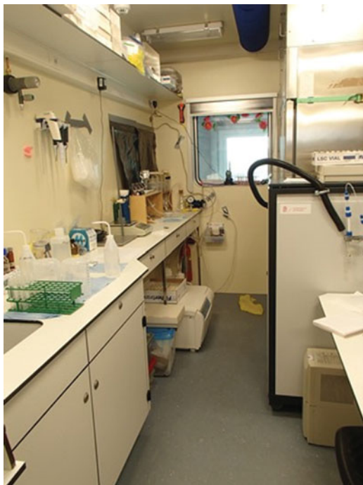
Fig. 12. Lab 3: set up for culturing using an open cabinet with plasma lamps that provide the daylight spectrum and fitted with a mass spectrometer (0–22°C). Photo: D. den Os
