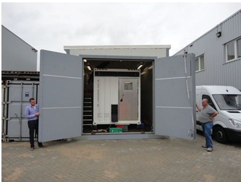
Fig. 9. The prototype container laboratory tested in a specially built cold store. Photo: M.G. Smit
