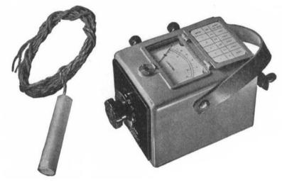
With this apparatus, soil moisture is determined by measuring the electrical resistance of gypsum cells buried in the soil, using a portable ohmmeter. The individual cells are manufactured from gypsum conforming to fine
