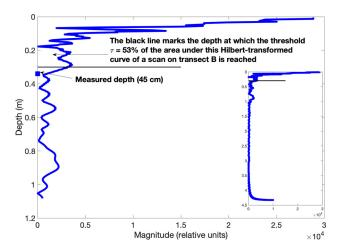
**Fig. 8.** An example Hilbert-transformed trace from 298 m along transect B (measured from transect start on climber's right) with the threshold applied. The upper bound of integration, which approximates the bottom of the debris layer, is shown as a black line. Only 256 samples are shown for clarity, but all 1024 are shown in the figure
