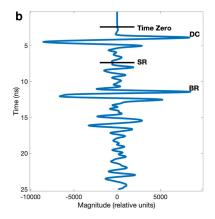
Fig. 7. (a) A radar profile collected with a raised 960 MHz antenna unit over the rock box in Fig. 3 that had three partitioned clast size sections, under which aluminum foil provided a strong bottom reflection (BR). Total debris depths were 28.6, 29.6 and 33.6 cm over the small debris, medium debris and large debris sections, respectively, and the DC and faint surface reflection (SR) are also marked. (b) The trace marked by the black line in (a), with the same labels as in (a).
