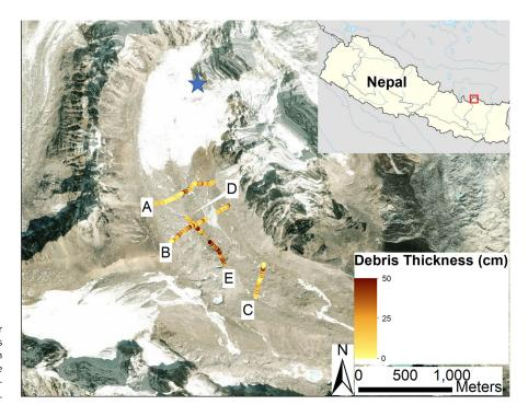
**Fig. 1.** GPR profiles A–E taken on Changri Nup Glacier with a 960 MHz antenna unit. The colorbar indicates debris depth determined by volumetric backscatter in GPR profiles. The star indicates the likely source of the debris ridge down the midline of the glacier's accumulation zone. Note the large ice sail intersecting transect B.
