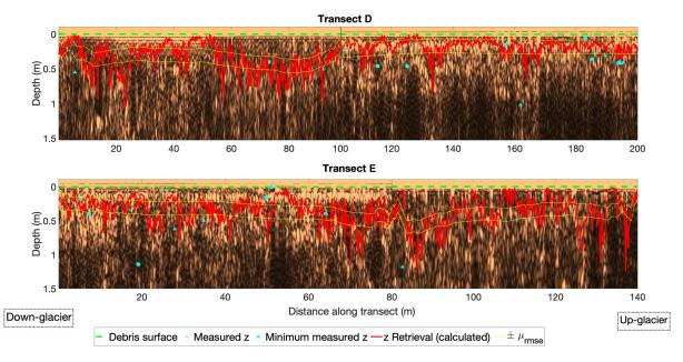
**Fig. 6.** Top 1.5 m of the Hilbert-transformed GPR data, GPR-based thickness retrievals (red) and ground-truth measurements ( $\bullet$  and  $\triangle$ ) along profiles over two along-glacier transects on Changri Nup Glacier, starting at their down-glacier ends. These profiles are much shorter than those in Fig. 5 and, for visual interpretation, are not stacked here. As in Fig. 5, z is thickness and a depth of 0 m is the debris surface.
