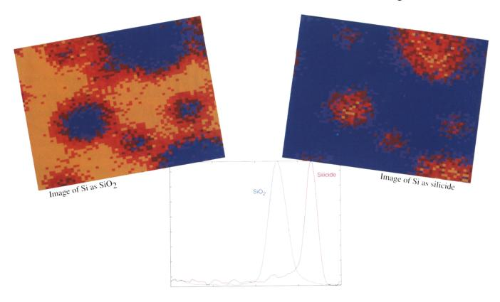
The 5600ci was used to image the silicon chemistry of a blistered thin film. Spectral data stored at each pixel were examined and two separate silicon chemical states were identified (bottom). The map was separated into two images -- Si as SiO<sub>2</sub>, and Si as silicide.
