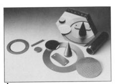
A Silicon Carbide Components: Morton Advanced Materials' CVD SILICON CARBIDE™ is available in preshaped components of many geometries having properties of a cubic (β) material. Morton's CVD process can produce bulk, free-standing substrates several square feet in area and up to 1 in. thick, or to customer specifications. Applications include nozzles, electronic packaging, high-temperature processing tools, seals, and wear parts. Circle No. 87 on Reader Service Card.
