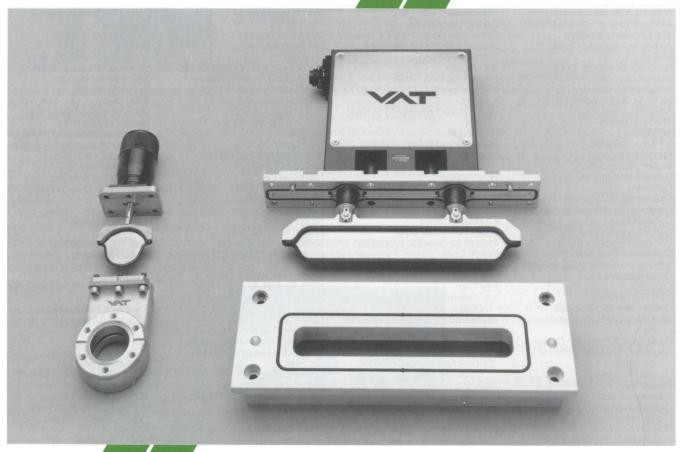
Because there is only one moving part with no cams or bearings under vacuum, MONOVAT valves operate virtually particle-free and maintenance-free typically far beyond a million cycles. They are available with circular or rectangular openings in a variety of sizes in aluminum or stainless steel.
