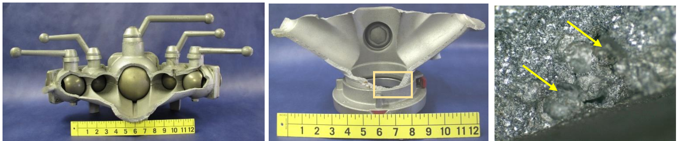
Figure 1. Several views of the ruptured hose manifold. Box in middle photograph shows location of right photograph as well as photographs in Figure 2. Right photograph shows voids in casting wall (arrows).
