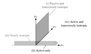
FIGURE 3. Regimes of interest in the parameter space: (i) the plane  $\mu_1 = 0$  is the passive transversely isotropic regime; (ii) the dashed line represents the active-only regime where  $\mu_2 = \mu_3 = 0$ ; (iii) the quarter cylinder is the nearly isotropic regime where neither  $\mu_2$  nor  $\mu_3$  is large; (iv) the remaining region is the fully active and transversely isotropic regime.
