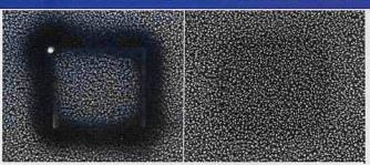
A silicon "grass" sample irradiated for 10 minutes before (left) and after (right) the use of Evactron Anti-Contaminator. 50kX - From Active Monitoring and Control of Electron Beam Induced Contamination by A. Vladar, M. Postek, & R. Vane., Proc. SPIE Vol. 4344 (2001), 835.
