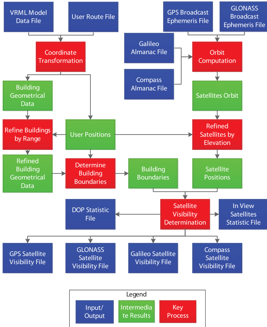
Figure 2. Software flowchart for satellite visibility determination.
