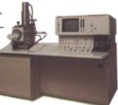
Images are sharp because the JSM-820 is equipped with computer controlled electron optics, a corrected field (C-F)
