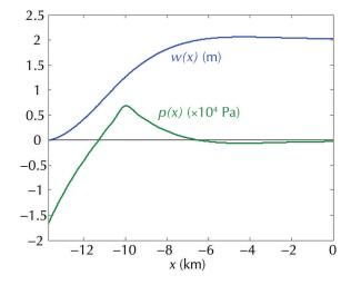
**Fig. 2.** Excess pressure, p(x) (green), and opening profile, w(x) (blue).
