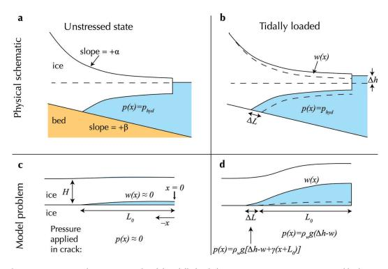
**Fig. 1.** (a, b) Schematic geometry under (a) unstressed and (b) tidally loaded cases. Water pressure, *p*, is assumed hydrostatic,  $p(x) = p_{hyd}$ , and both surface slope and bed slope are assumed constant near the grounding line. (c, d) Modeled crack-opening problem corresponding to the (c) unstressed and (d) tidally loaded cases.
