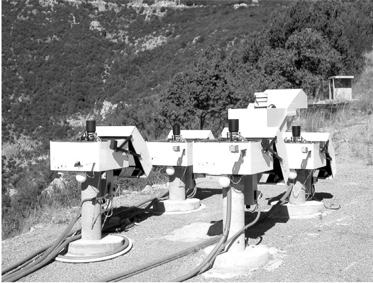
**Figure 1.** HATNet station at FLWO, Arizona, hosting HAT-5, 6, 7 and HAT-10, plus TopHAT (in the background). The clam-shell domes are normally closed in the daytime, and protect all the equipment inside: the Canon 200mm f/1.8 lenses,  $4K \times 4K$  CCDs and horseshoe mounts.
