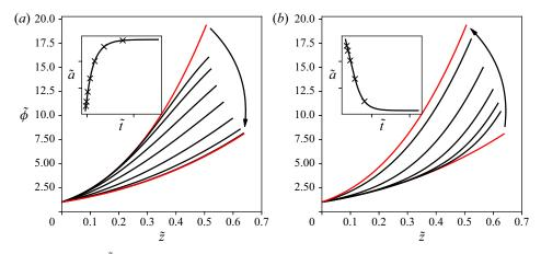
Figure 9. Change of  $\tilde{\phi}$  in response to changes in evaporation rate  $\tilde{q}$  during swelling (a) and shrinking (b); corresponding to the first swelling–shrinking cycle in figure 8. Steady states are shown by the outer red lines, the inner black lines represent transients at times shown as crosses in the insets.
