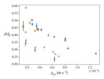
Figure 5. Overview of the steady-state data from datasets obtained under consistent experimental conditions for constant *H*. Blue circle – dataset B (H = 2.6 cm), orange diamond – dataset D (H = 5.2 cm), green triangle – dataset E (H = 10 cm), red fatplus – dataset F (H = 20 cm), see table 1 for further details.
