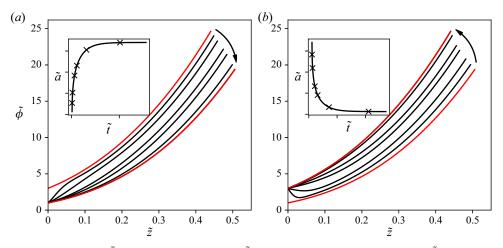
Figure 10. Changes of  $\tilde{\phi}$  in response to changes of  $\tilde{H}$  with constant  $\tilde{q}$  during (a) swelling ( $\tilde{H}: 2 \rightarrow 0$ ) and (b) shrinking ( $\tilde{H}: 0 \rightarrow 2$ ). Steady states are shown by the outer red lines, the inner black lines represent transients at times shown as crosses in the insets.
