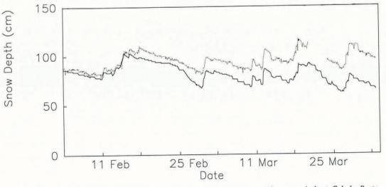
Fig. 7. Measured (--) and simulated (-) snow depth during the second test period at Col de Porte.
