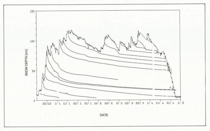
Fig. 1. Snow depth and compaction of each layer observed during the 1986-87 winter at Col de Porte. Missing snow-depth data are shown by the dashed line.
