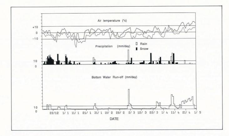
Fig. 2. Maximum and minimum daily temperature, snow and rain precipitation, and bottom-water run-off observed during the 1986-87 winter at Col de Porte.
