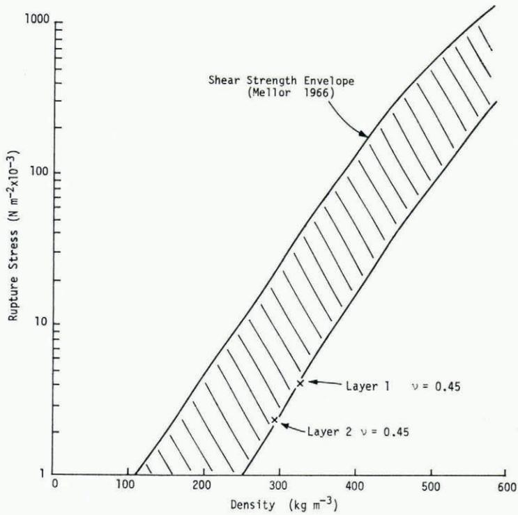
Fig. 5. Shear strength of snow.
