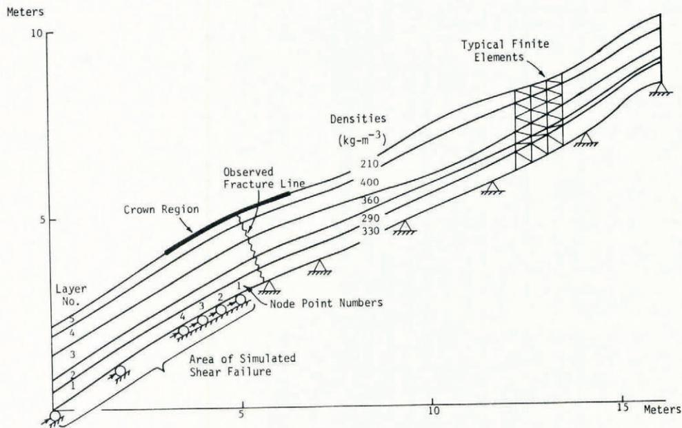
Fig. 1. Schematic of a realistic snow-pack.
