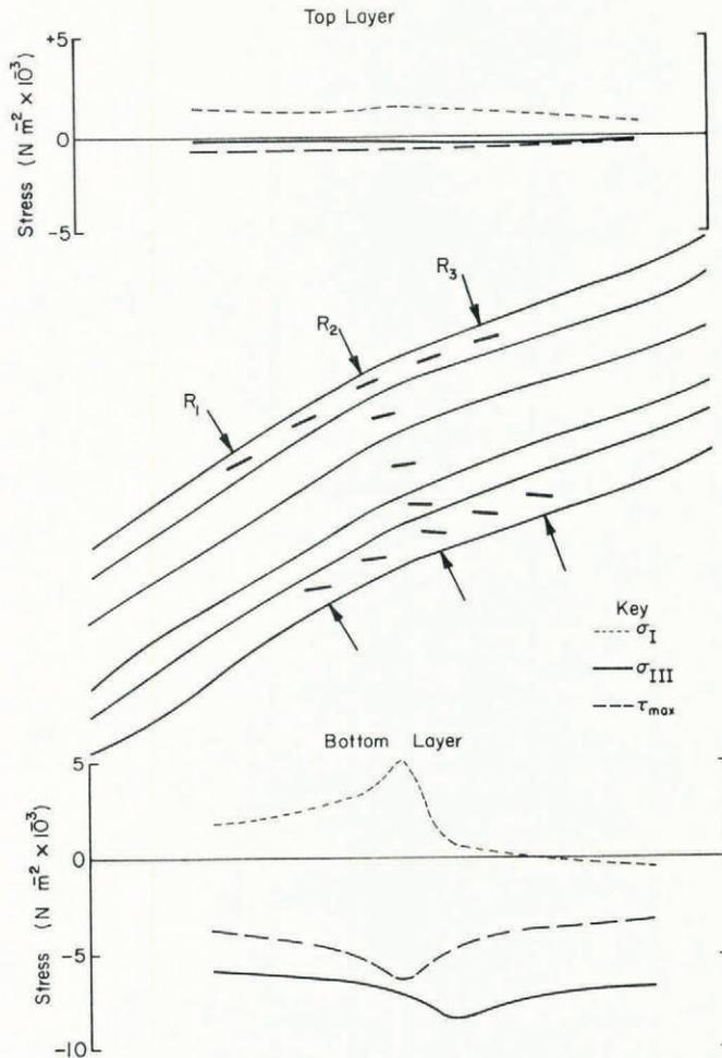
Fig. 7. Principal stress magnitudes and directions in the crown region, simulated shear failure,  $\nu = 0.25$ .
