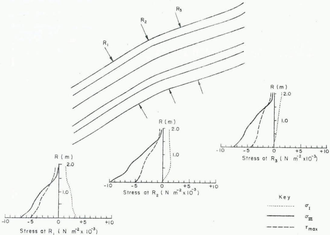
Fig. 8. Principal stresses in the crown region, simulated shear failure,  $\nu = 0.25$ .
