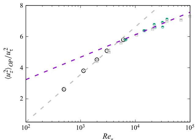
Figure 12. Magnitude of outer peak of axial velocity variance as a function of  $Re_\tau$ . Lines and symbols as in tables 1 and 3. The dashed grey line marks the DNS data fit,  $\langle u_z^2 \rangle_{OP}^+ = 1.33 \log Re_\tau - 5.61$ , and the purple line denotes the logarithmic fit given by Pullin *et al.* (2013).
