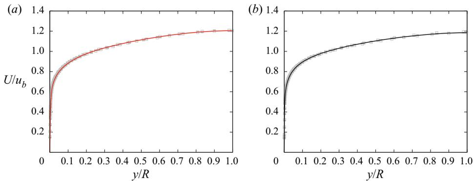
Figure 5. Mean velocity profiles in outer scaling. Data of flow case DNS-E (a) are compared with SuperPipe data at  $Re_\tau = 3328$  and  $Re_\tau = 3334$ , and data of flow case DNS-F (b) with SuperPipe data at  $Re_\tau = 5411$  and  $Re_\tau = 6617$ .
