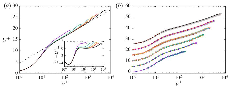
Figure 3. Inner-scaled mean velocity profiles obtained with our DNS (a), and compared with previous DNS and experiments (b). Deviations from the assumed logarithmic wall law,  $U_{log}^+ = \log y^+ / 0.387 + 4.53$ , are highlighted in the inset of panel (a). For greater clarity, profiles in panel (b) are offset in the vertical direction by five wall units steps. Lines denote present DNS data, with colour code as in table 1, and symbols denote data from other authors, as in table 3.
