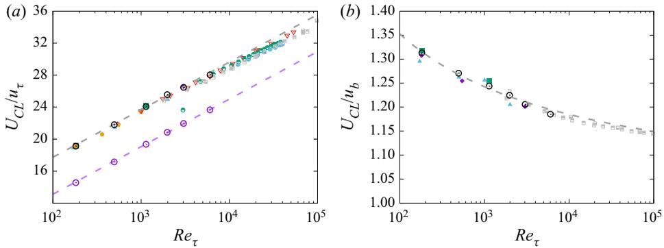
Figure 7. Mean pipe centreline velocity ( $U_{CL}$ ) expressed in inner (a) and in outer (b) units. The dashed grey line corresponds to a fit of the DNS data. The DNS data are shown as circle symbols, and the corresponding logarithmic fits are shown as thick dashed lines. Purple lines and symbols are used for the bulk velocity,  $u_b$ . For the nomenclature of other symbols, refer to [table 3](#).
