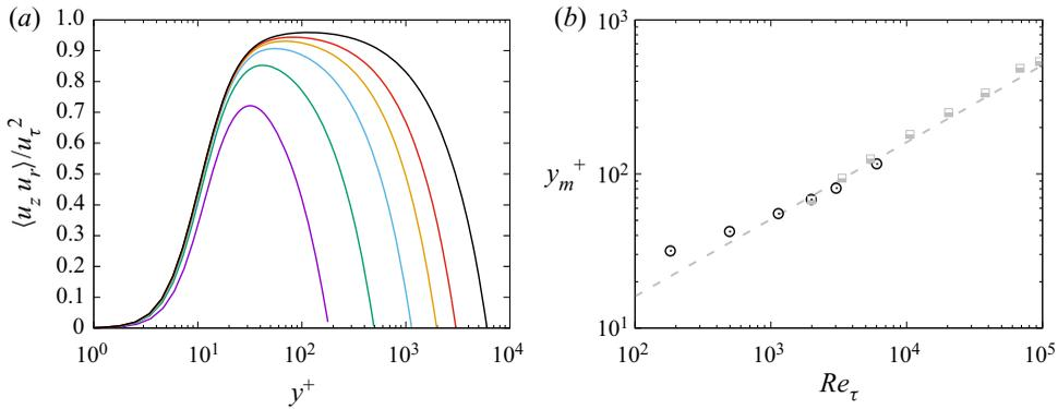
Figure 9. Distributions of turbulent shear stress (a) and its peak position at various  $Re_\tau$  (b). In panel (b) the circles denote the present DNS data, the squares the data of Hultmark *et al.* (2013), as processed by Chin *et al.* (2014), and the dashed line the theoretical estimate (3.8). For colour codes in DNS data, see table 1.
