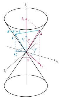
Figure 2. Constant-frequency cone in wavevector space displaying the spherical coordinates used in the representation (3.1a,b) of the wavevectors k and k'. Scattering transfers energy between IGWs with the same frequency; hence their wavevectors k and k' lie on the same cone. The wavevector K = k' - k of the geostrophic mode inducing the scattering is also shown.
