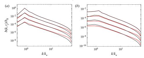
Figure 7. Log-log representation of the IGW spectrum in figure 6(c), i.e. for  $\omega = 2f$  and Ro = 0.049 obtained from the kinetic equation (red lines) and Boussinesq simulations (black lines); (a)  $b_+(k,t) = b(k,t)$ , corresponding to the upper nappe of the dispersion-relation cone, (b)  $b_-(k,t) = b(-k,t)$ , corresponding to the lower nappe. The curves correspond to the times shown in figure 6(c) and are successively shifted downwards by half a decade for clarity.
