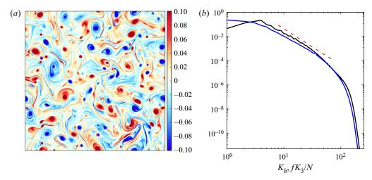
Figure 5. Vertical vorticity on the horizontal plane z = 0 (a) and kinetic energy spectrum of the initial geostrophic flow (b). Both horizontal (black line) and vertical spectra (blue line) are shown, with a  $K^{-3}$  power law (indicted by the dashed line).
