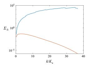
Figure 4. Total cross-sections for same-nappe and across-nappe transfers  $\Sigma_+(k)$  (blue line) and  $\Sigma_-(k)$  (red line) defined in (3.7) for  $\omega=2f$ , N/f=32, Ro=0.099 and the quasigeostrophic-flow energy spectrum described in § 4.1.
