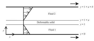
FIGURE 1. Schematic of the flow geometry in dimensionless coordinates. The plates at y = 0 and y = 1 + a + b are moving with dimensionless speeds 1 and  $V_r$ , respectively. The fluids exert a shear stress at the fluid–DS interface, leading to deformation of the DS and coupling between the base-state fluid motion and perturbations in the DS, which affects the stability of the flows.
