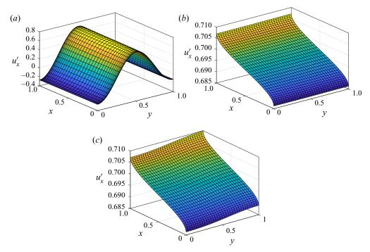
FIGURE 4. The normalised horizontal perturbation displacement of the DS for the remaining three modes at a=0.6, b=1,  $\Gamma=0.57$ ,  $\mu_r=0.5$ , k=0.029,  $\Sigma_1=1$ ,  $\Sigma_2=1$  and  $V_r=0$ . Panels (a-c) are for the second, third and fourth modes, respectively, which are all stable. The designations first, second, third and fourth modes refer to the number of the mode when the eigenvalues arranged in the descending order of the imaginary part similar to table 2.
