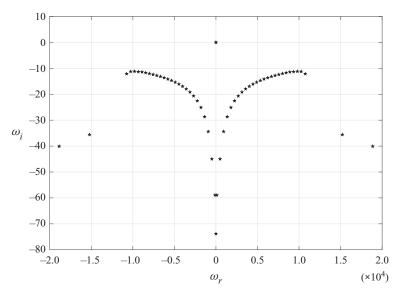
FIGURE 8. The eigenvalue spectrum at Re = 0.1, a = 0.1, b = 1,  $\mu_r = 0.5$ ,  $V_r = 0$ ,  $\Gamma = 0.05$ , k = 0.05,  $\Sigma_1 = 1$  and  $\Sigma_2 = 1$ . The shear waves arising due to the interaction of the fluids and DS are symmetrically distributed about  $\omega_r = 0$  line. The unstable viscous mode of instability,  $\omega = 0.013500 + 0.000727i$  is located on the symmetry line of the spectrum.
