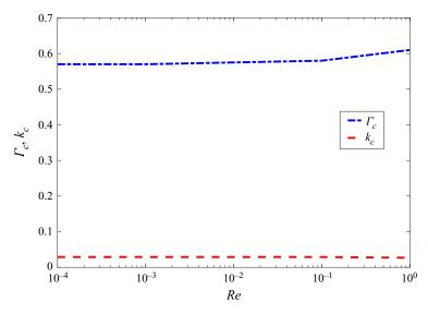
FIGURE 9. The variation of  $\Gamma_c$  and  $k_c$  with Re at a=0.6, b=1,  $\mu_r=0.5$ ,  $V_r=0$ ,  $\Sigma_1=1$  and  $\Sigma_2=1$ . The figure illustrates the stabilising effect of inertia on the viscous instability. The viscous instability remains the dominant mode of instability for Re<1.
