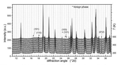
FIG. 7. Powder XRD patterns of Pb-lawsonite (T = 298 to 498 K) showing the phase transition from space group Pbnm to Cmcm around 450 K. The XRD patterns were smoothed and vertically offset to enhance the visibility of the small diffraction peaks. Arrows indicate a number of weak, critical reflections and their indices.
