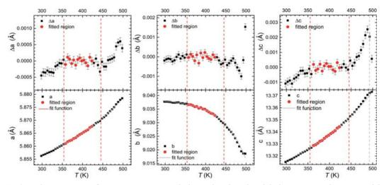
FIG. 9. Lattice parameters *a*, *b*, *c* versus temperature. The lower plots show the original parameters and an exponential decay function fitted to the central (marked) data points. The upper plots show the differences between the fit functions and the data points. The dashed lines mark the transition temperatures that were obtained from the principal component analysis plus subsequent cluster analysis of the diffraction patterns.
