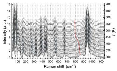
FIG. 4. Temperature-dependent Raman spectra of Pb-lawsonite from 298 to 573 K showing the vibrations of the  $Si_2O_7$  groups and AlO<sub>6</sub> octahedra as well as lattice vibrations. Spectra are vertically offset. The bold line at  $\approx$ 790–860 cm<sup>-1</sup> indicates the maximum of the  $\gamma$ -OH vibrational band.
