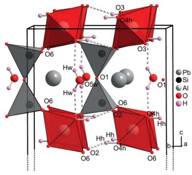
FIG. 1. Part of the unit cell of Pb-lawsonite, space group *Pbnm*, at room temperature. Broken grey lines indicate H bonds with H<sup>...</sup>O distances of 1.95 to 2.06 Å.
