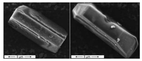
FIG. 2. Scanning electron microscopy – secondary electron images of two larger Pb-lawsonite crystals synthesized from PbAl<sub>2</sub>SiO<sub>x(7-8)</sub> glass and excess water in a piston cylinder experiment at 600°C and 4 GPa.
