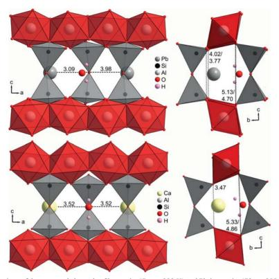
FIG. 12. Comparison of the structural channels of lawsonite (*Pmcn*, 233 K) and Pb-lawsonite (*Pbnm*, 298 K) hosting the Ca/Pb cation and the H<sub>2</sub>O molecule, in two different orientations. Numbers denote the interatomic distances in Å. Note the straightened Si–O–Si angle in Pb-lawsonite, resulting in a more circular cross-section of the channel.
