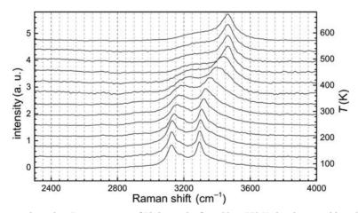
FIG. 3. Temperature-dependent Raman spectra of Pb-lawsonite from 83 to 573 K showing stretching vibrations of the hydroxyl groups and the H<sub>2</sub>O molecule. Spectra are vertically offset and smoothed only for presentation.
