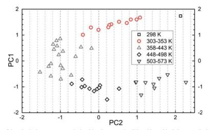
FIG. 6. Results of the principal component analysis with subsequent Euclidean hierarchical cluster analysis of the Raman spectra of Pb-lawsonite at different temperatures.
