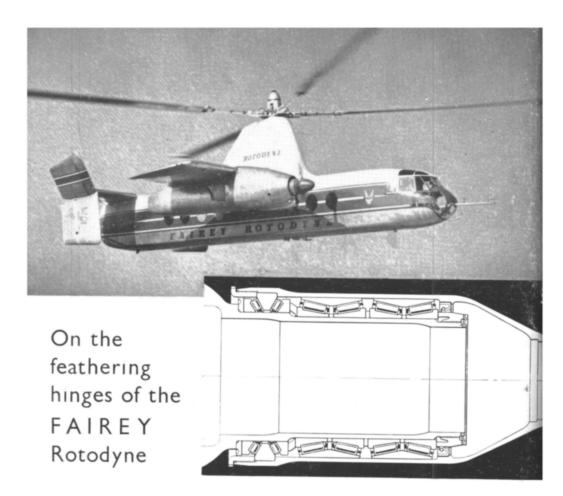
On this, the world's first vertical take-off airliner, Timken tapered-roller bearings are used in important situations
