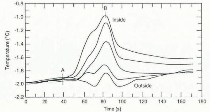
Fig. 8. Basal temperatures from inside to outside of DH skis.  $T_0 = -2^\circ\text{C}$ ;  $v_{\text{max}} \approx 9 \text{ m s}^{-1}$ ; parallel run down gentle slope with load of  $N/2$  on soft, fresh snow.
