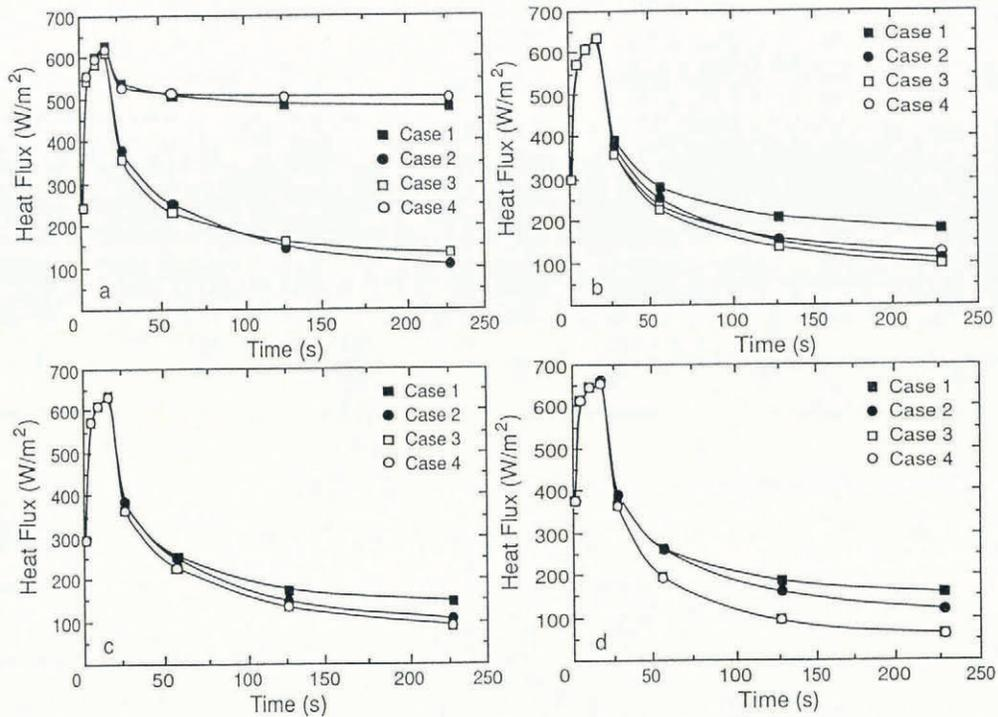
Fig. 13. Computed heat flux versus time for four transverse positions and four cases of different materials as described in the text.  $T_0 = -5^\circ\text{C}$ ;  $v = 18 \text{ m s}^{-1}$ ; load  $N/2$ . (a) 3 mm from edge; (b) 100 mm from edge; (c) 25 mm from edge; (d) on center line, 37 mm from edge.
