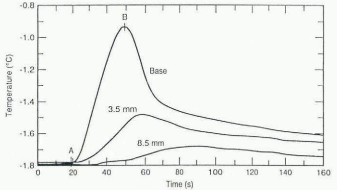
Fig. 11. Vertical temperature profile of DH ski showing basal, 3.5 and 8.5 mm responses.  $T_0 = -1.8^\circ\text{C}$ ;  $v_{max} \approx 9 \text{ m s}^{-1}$ ; parallel run down gentle slope with load  $N/2$  on soft, fresh snow.
