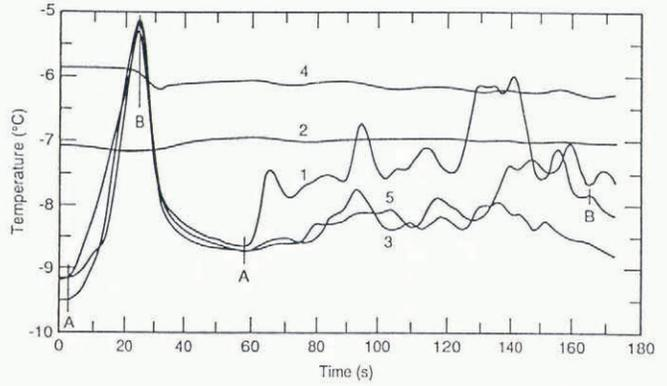
Fig. 10. Temperatures in plastic ski. 1, 3 and 5 are on base in left, middle and right side. 2 is 3.8 mm above and 4 is 9.7 mm above base.  $T_0 = -9.3^\circ\text{C}$ ;  $v_{max} \approx 6 \text{ m s}^{-1}$ ; parallel run down gentle slope with load  $N$  on hard-packed snow then up Poma lift at  $\approx 2 \text{ m s}^{-1}$ .
