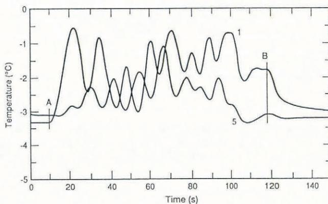
Fig. 7. Basal temperatures on left and right sides of plastic ski during many turns. 1 is the inside and 5 is the outside of the ski.  $T_0 = -3.2^\circ\text{C}$ ;  $v_{\text{max}} \approx 6 \text{ m s}^{-1}$ ; wide, smooth turns with load of  $N/2$  on soft, fresh snow.
