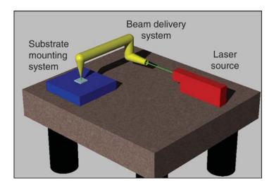
Figure 1. Schematic illustration of a laser direct-write system. The basic components of an LDW system are (left to right) a substrate mounting system, a beam delivery system, and a laser source. Motion control of either the beam delivery system or the substrate mounting system is typically accomplished using computer-assisted design and manufacturing (CAD/CAM) integrated with the laser source.
