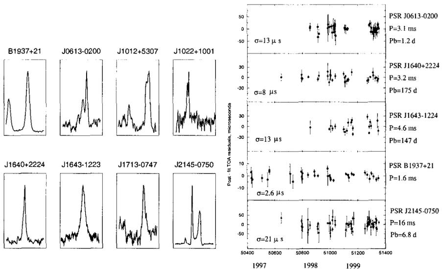
Figure 1. Pulse profiles of millisecond and binary pulsars at 0.6 MHz, observed with 64-m antenna at Kalyazin (*left panel*) and the TOA residuals after fit of pulsar spin, astrometric, and Keplerian parameters (*right panel*).
