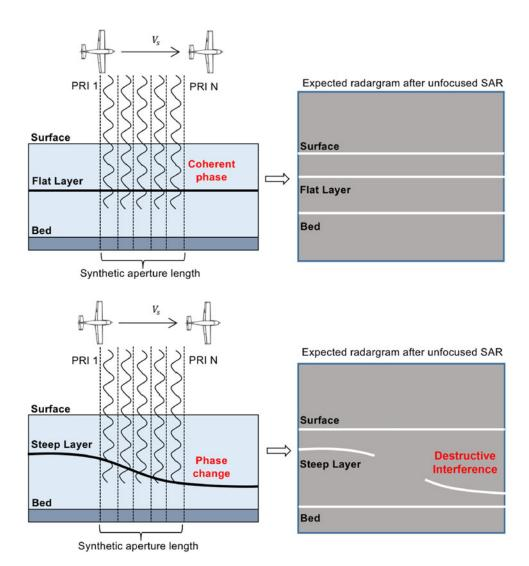
Fig. 1. Comparison of unfocused processing effects on flat (above) and sloping (below) subsurface layers. The difference in instantaneous phases within the coherent summation window can destroy steep layers (see also Holschuh and others, 2014).
