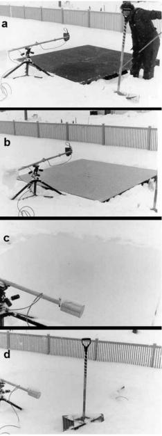
**Fig. 2.** Photographs of the black base taken over a 5 hour period during a snowfall. The snow depths were (a) 0 cm, (b) 0.5 cm, (c) 3 cm and (d) 8 cm.
