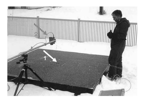
Fig. 1. The experimental set-up consisted of a  $2.4 \text{ m} \times 2.4 \text{ m}$  black plywood base with a detector mounted in the center (arrow 1) that measured transmitted irradiance. Incident and reflected irradiance were measured using a second detector that was mounted on a tripod (arrow 2).
