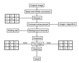
Fig. 2. Schema of the image treatment program.
