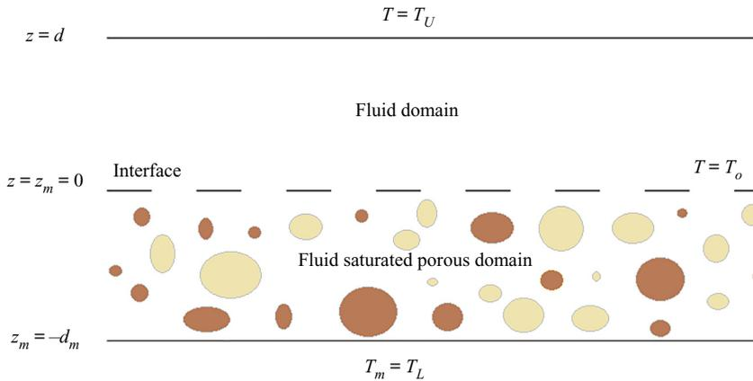
Figure 1. Schematic diagram of the system under consideration.
