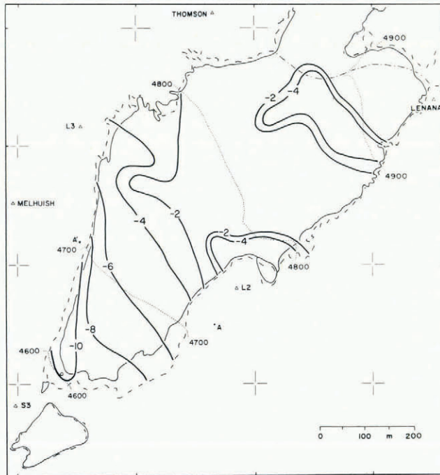
Fig. 3. Changes in ice thickness, March 1982 minus February 1978, in metres, as determined from the two airborne mappings. Ice rim in 1982 is shown as solid, and in 1978 as broken line. 1978 height contours are entered as thin dotted lines.
