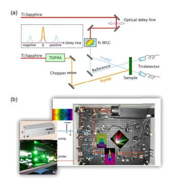
**Figure 2.** (a) Schematic optical layout of a typical ultrafast TA setup that features a tunable pump (delivered by a femtosecond optical parametric amplifier) and a broadband WLC probe (generated by focusing a small portion of the Ti:sapphire regenerative amplifier output in a transparent nonlinear crystal). (b) The CDP ExciPro femtosecond pump–probe system that operates in our ultrafast spectroscopy laboratory at USTC<sup>[15]</sup>.
