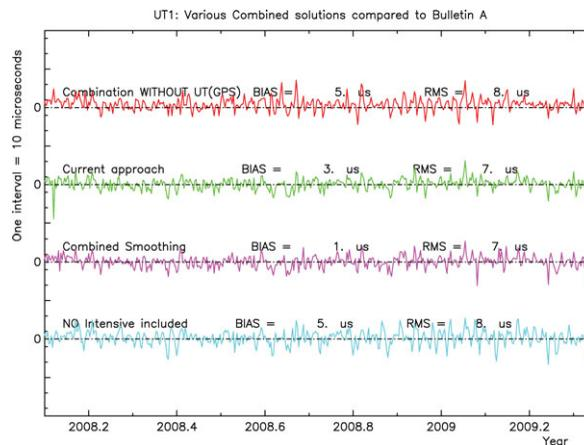
**Figure 1.** Comparisons of different UT1 combined series using or not UT(GPS). It appears that the contribution of GPS LOD either by the direct integration of LOD(GPS) referred as Current approach, or when applying the Combined Smoothing leads to a small improvement in the WRMS compared to the usual solution. We can remark that the inclusion of Intensive sessions does not significantly improve the final combined UT1 solution.
