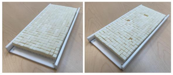
Figure 3. Fully assembled prototype (left) and prototype where four sensors have been triggered by high pressure (right)
