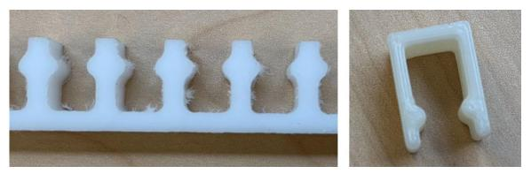
Figure 2. Part of a CNC machined strip of base parts (left) and a 3D printed switch (right)
