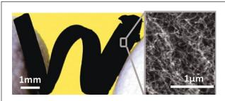
Flexible intertube carbon nanotube material, with scanning electron micrograph (inset). Reproduced with permission from *Science* **330** (6009) (2010) DOI: 10.1126/science.1194865; p. 1364. © 2010 AAAS.
