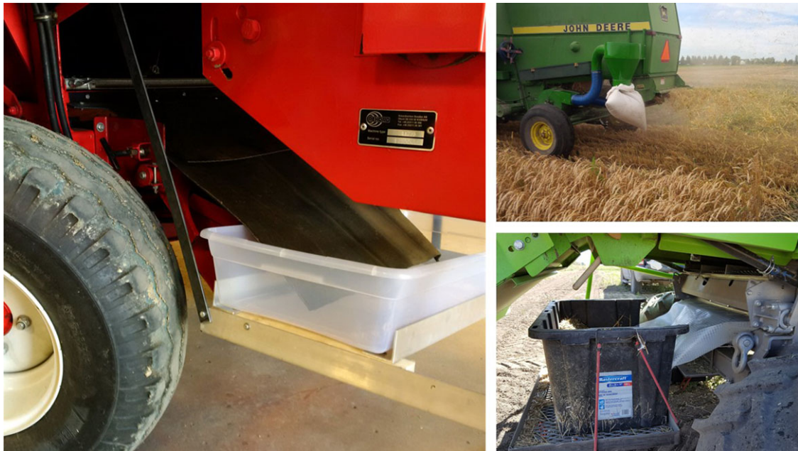
Figure 1. Examples of chaff collection systems used on different plot combines in the study conducted from 2016 to 2018 to investigate crop rotation maturity, harvest management and harvest weed seed control effects on wild oat populations. Each combine has unique chaff and straw spreading setups and so each chaff collection system was unique to individual locations. These are three examples of systems used in this study.
