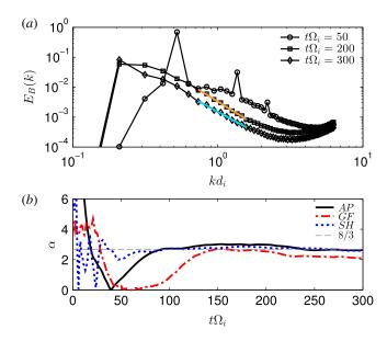
FIGURE 2. (a) Magnetic power spectra for the AP run, at different times, with the powerlaw fit. (b) The time evolution of the spectral index  $\alpha$  obtained from the fits for the three runs. The horizontal line marks the scaling exponent value 8/3.
