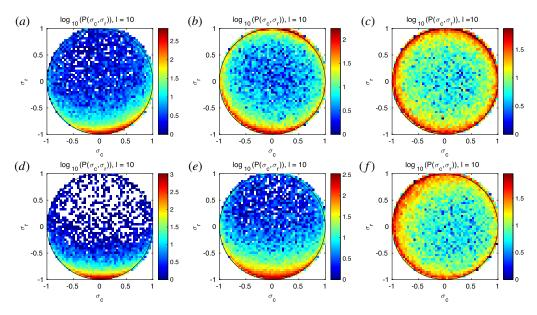
FIGURE 8. Distribution of fluctuations as a function of residual energy  $\sigma_r$  and cross-helicity  $\sigma_c$ , for the cases AP (a,d), SH (b,e) and SH2d (c,f). Distribution functions have been calculated for the periods  $t\Omega_i = 40-60$  in (a-c) and  $t\Omega_i = 280-300$  in (d-f), with lag  $l = 10d_i$ .
