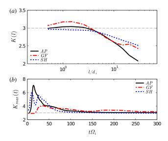
FIGURE 5. (a) The scale dependence of the kurtosis for the  $B_x$  increments for all three 3-D simulations, at the final time of the simulation. (b) The time evolution of the maximum of the scale-dependent kurtosis across all scales, again for the  $B_x$  increments.
