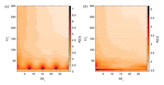
FIGURE 6. Time dependence of the scale-dependent kurtosis for the AP case (a) and SH case (b). Note that at early times in the AP case high kurtosis is associated with multiples of the sheet separation scale.
