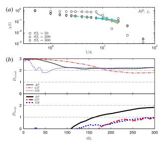
FIGURE 7. (a) The cancellation functions of the  $j_z$  component,  $\chi(l)$ , at three different times, for the AP run. Power-law fits are indicated in two ranges of scale above and below the break at  $l_{\star}$ . (b) The time evolution of the fractal dimension  $D_{small}$  (upper window, thin lines) and  $D_{large}$  (lower window), for all three runs.
