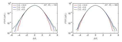
FIGURE 3. Examples of the PDFs of the longitudinal field increments of the x component,  $\Delta B_x$ , at three different scales (different colours), estimated at two times in the simulation, for the anti-parallel case. The weak scale dependence is highlighted by the comparison with a reference Gaussian (dashed lines). A similar behaviour is observed at all times, for all the field components, and for all simulation cases (not shown).
