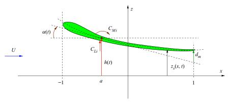
Figure 1. Schematic of foil motion (non-dimensional).
