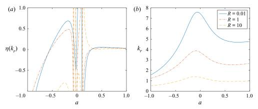
Figure 14. Efficiency at  $k = k_r$  (a) and the corresponding  $k_r$  (b) versus a for a pitching motion with  $a_0 = 2^\circ$  and  $C_{D0} = 0.05$ , for S = 10 and three values of R.
