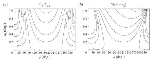
Figure 17. Thrust (a) and efficiency (b) enhancement by adding a pitching motion about the leading edge (a=-1) of amplitude  $a_0$  and phase shift  $\phi$ , in relation to the thrust and efficiency of the heaving-only motion,  $\bar{C}_{Th} \simeq 0.378$  and  $\eta_h \simeq 0.4$ , respectively, with  $h_0 = 0.02$  and  $C_{D0} = 0.05$ , for a foil with R = 0.01 and S = 130, and a reduced frequency k = 6.9. The contour values in (b) are for  $(\eta - \eta_h) \times 100$ .
