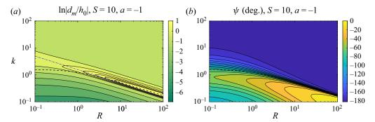
Figure 4. As in figure 3 but as a function of reduced frequency k and mass ratio R for a plate with stiffness S = 10. The dashed lines correspond to the first natural frequency of the system  $k_r$  that minimizes  $|F_2|$ , while the dashed-and-dotted line is  $k_{r0}$  ( $\propto R^{-1/2}$ ) given by (3.5), valid for for  $R \gg 1$ .
