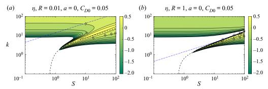
Figure 9. Efficiency  $\eta$  as a function of frequency and stiffness for a heaving foil with a=0, R=0.01 (a) and R=1 (b), and using  $h_0=0.02$  with  $C_{D0}=0.05$ . The dashed lines correspond to the first natural frequency of the system  $k_r$  that minimizes  $|F_2|$ , while the dashed-and-dotted line is  $k_{r0}$  given by (3.5). Areas with  $\eta<-1$  have been whited out.
