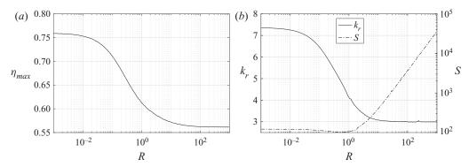
Figure 16. Maxima in the efficiency versus the mass ratio (a) and the corresponding values of the stiffness and frequency (b) for a pitching motion about the leading edge with  $a_0 = 2^{\circ}$  and  $C_{D0} = 0.05$ .
