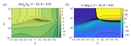
Figure 5. Amplitude of the flexural component of the deflection (a) and its phase (b) as a function of reduced frequency k and the location a where the heaving motion is imposed to a plate of stiffness S = 10 and mass ratio R = 0.01. The dashed lines correspond to the first natural frequency of the system  $k_r$  that minimizes  $|F_2|$ .
