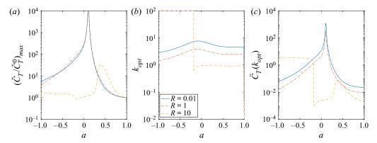
Figure 8. Maxima of the thrust enhancement (a), optimal frequency (b) and thrust at the optimal frequency (c) versus the pivot point location a for three values of the mass ratio R, when the stiffness of the heaving foil is S = 10.
