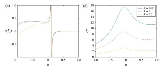
Figure 10. Efficiency at  $k = k_r$  as a function of the pivot point location (a) and the corresponding  $k_r$  (b) for S = 50 and three values of R, for a purely heaving motion with  $h_0 = 0.02$  and  $C_{D0} = 0.05$ .
