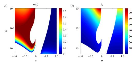
Figure 15. Efficiency at  $k = k_r$  (a) and and the corresponding frequencies (b) in the stiffness-pivot point location plane for a purely pitching motion with  $a_0 = 2^{\circ}$  and  $C_{D0} = 0.05$  for R = 0.01. Areas with negative or singular efficiency have been whited out.
