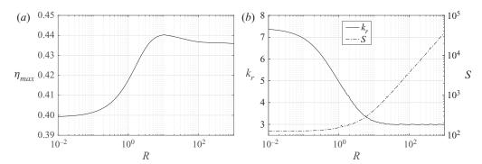
Figure 12. Maxima in the efficiency versus the mass ratio for a heaving motion pivoting at the leading edge (a) and the corresponding values of the stiffness and frequency (b). Here  $h_0 = 0.02$  and  $C_{D0} = 0.05$ .
