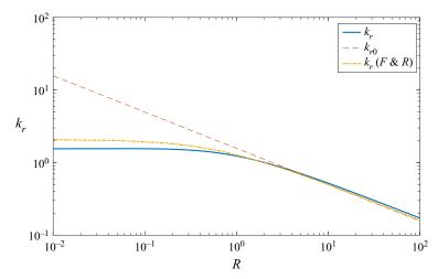
Figure 2. Natural frequency  $k_r$  obtained by minimizing  $|F_2|$  as a function of R for S = 10 and a = -1 (continuous line) compared with the first natural frequency computed by Floryan & Rowley (2018) (dashed-and-dotted line). The dashed line is  $k_{r0}$  from (3.5).
