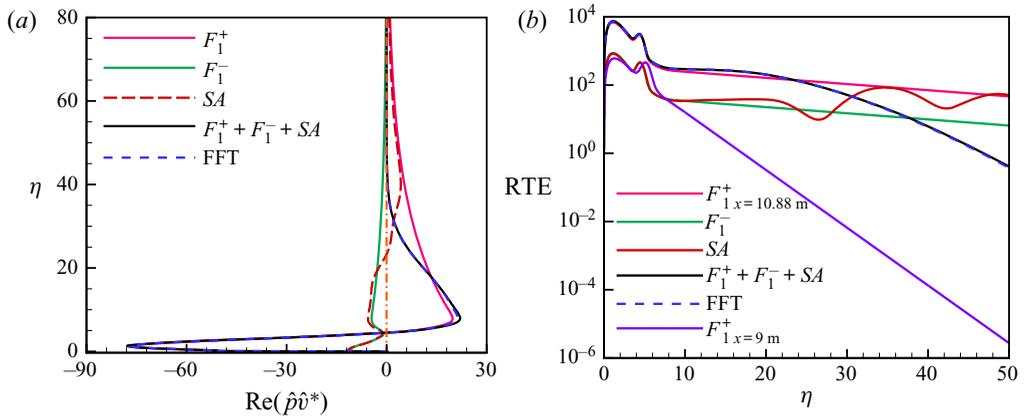
Figure 7. (a) Variation of the real component of pressure work along the boundary layer at  $x = 10.88$  m. (b) Rate of change of total disturbance energy for the supersonic mode computed at  $x = 10.88$  m compared with the second mode  $F_1^+$  at  $x = 9$  m.
