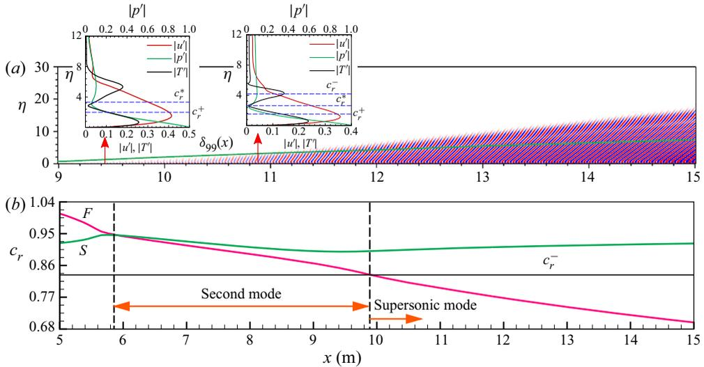
Figure 1. (a) Disturbance pressure field obtained from DNS and insets showing LST eigenfunctions for the second mode and the supersonic mode. Here  $c_r^-$  and  $c_r^+$  correspond to the phase speed of the slow and the fast acoustic waves, respectively, and  $c_r^*$  marks the critical layer. (b) Variation of the phase speeds of the fast mode  $F$  and the slow mode  $S$  along the flat plate showing the regions of the second mode and the supersonic mode.
