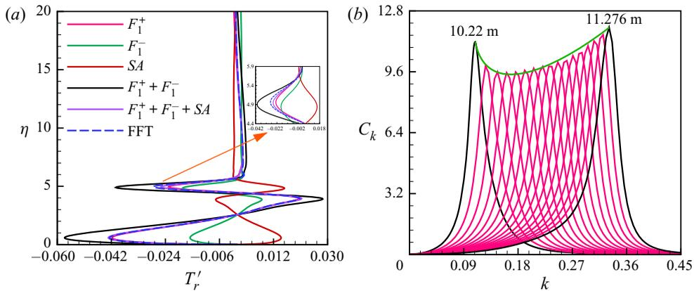
Figure 4. (a) Comparison of the real component of disturbance temperature obtained from BOD with FFT data at  $x = 10.22$  m. (b) Variation of the projection coefficient for the  $SA$  branch as a function of the continuous spectrum parameter  $k$ .
