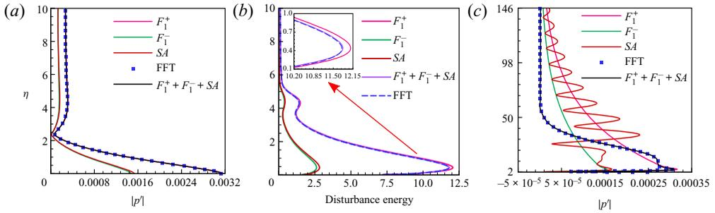
Figure 5. Variation of (a) amplitude of projected disturbance pressure and (b) total disturbance energy computed using Mack's energy norm along the boundary layer at  $x = 10.88$  m. (c) The projected amplitude profile of  $p'$  outside the boundary layer.
